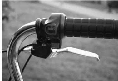
Attach brake cable to brake lever and connect to calipers.
