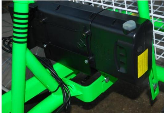
The Lithium Ion battery can be easily charged using the automatic charger connection on the end of the battery case Battery should be fully charged overnight before use.
